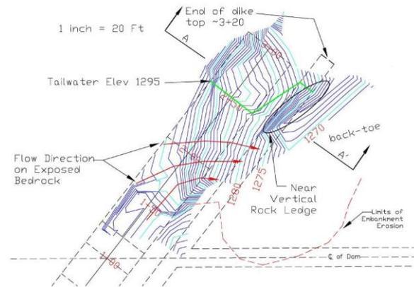
Figure 7 – Sugar Creek L-44 Plan of Erosion Damage
