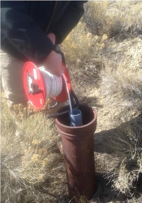
Photo 3: Standpipe Piezometer
