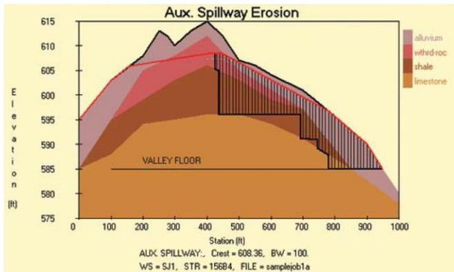
**Figure 3 – SITES Output of Predicted Erosion**
