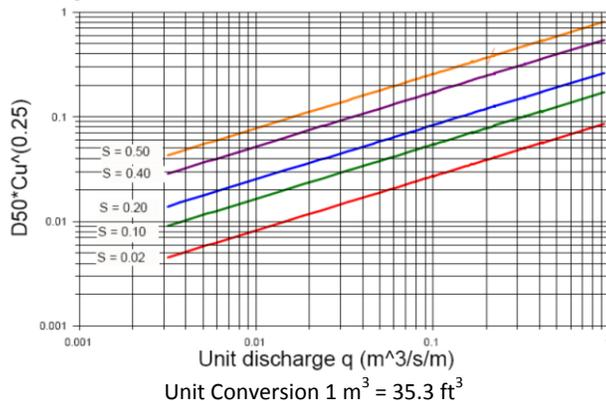
Figure 1 – Erosion Potential of Cohesionless Soil
