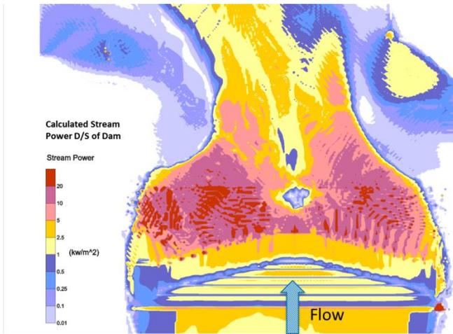
Figure 5 – CFD Model Estimated Stream Power
