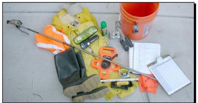
Photo 4: Typical inspection equipment.
