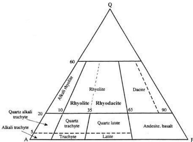
Figure 4 - QAP Diagram for Extrusive Rock
