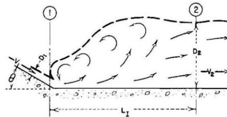
**Figure 14: Type I Hydraulic Jump on Horizontal Apron**
