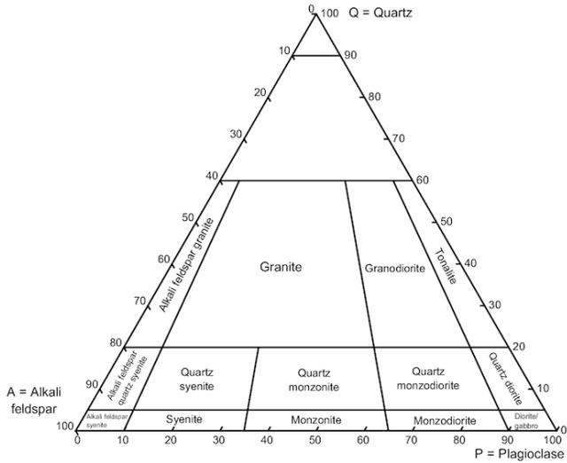
Figure 3 - QAP Diagram for Intrusive Rock
