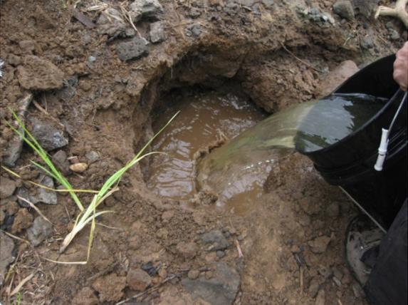
Photo 5: Flushing of sinkhole at Fish Lake, CO
