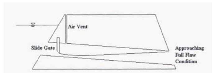
Figure 2: Air vent downstream of a slide gate
