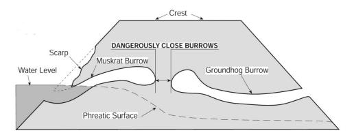
Heavy wire fencing laid flat against the slope and extending above and below the water line can also be effective. Eliminating or reducing aquatic vegetation along the shoreline will discourage muskrat habitation. Where muskrats have inhabited the area, trapping is usually the most practical method of removing them.
